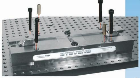
Unlike competitors' vises which must be awkwardly lifted up to load over pins or keys for alignment, the Stevens Two-Station Vise may be slid into position. Pull dowels are inserted from the top to align with bushings in the Stevens Subplate below.
